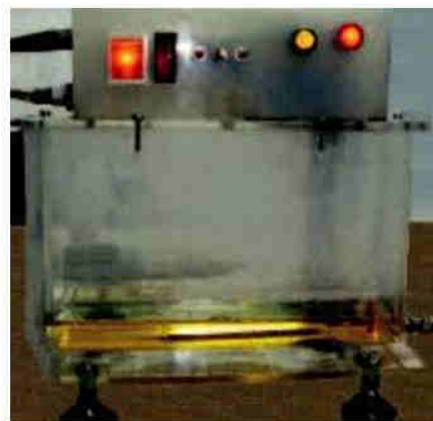
Figure1. Transesterification system used for the production of HOME
